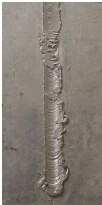
Figure 2. Cropped Image of Friction Stir Welded joint
