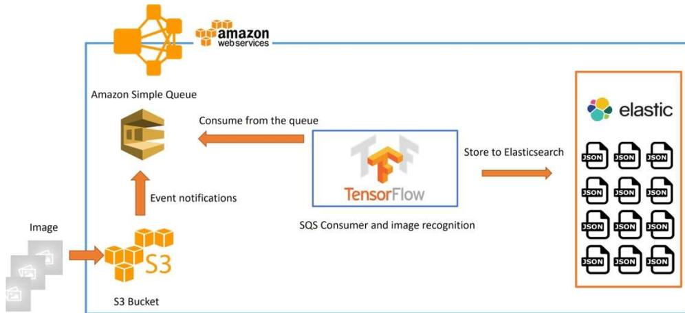
Figure 4 Image classification using sensor flow
