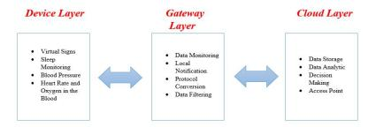
Figure 2. Architecture Block Diagram of IoMT
