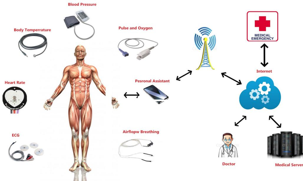
Figure 4. Illustration Architecture of Remote Patient Monitoring System
