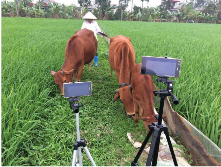
Figure 4. Recording for building the labelled data objects. The videos are synchronized with the acceleration data in order stick labels to the acquired data.
